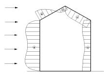
where  $C_p$  is wind surface pressure coefficient (empirical); it depends on wind direction, orientation of the building surface, ...  $C_p$  = -1.4 to 1.4
